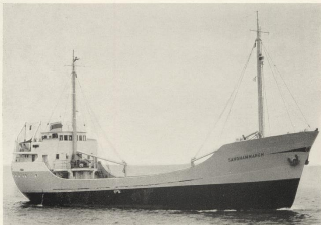
MV SANDHAMMAREN, built 1959, equipped with an engine of type 6 FD 300 MVH and a propeller device of type HR 131 F.
