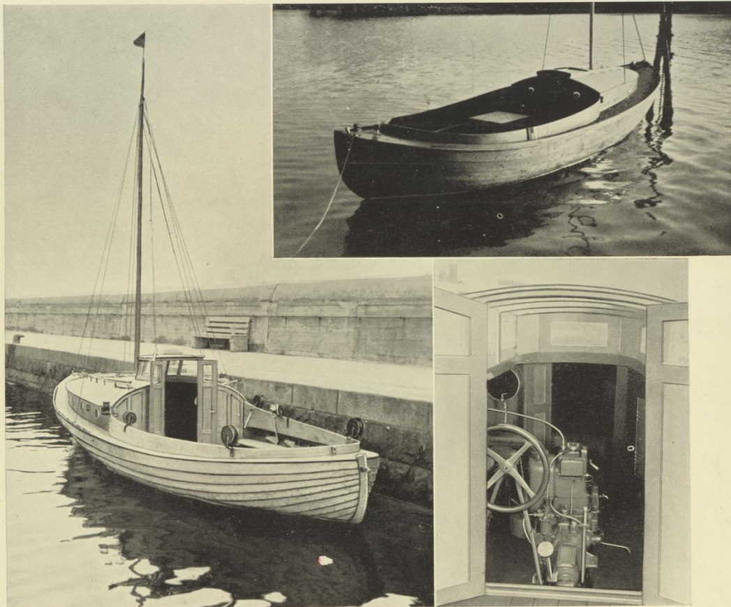
The above illustrations show some small fishing boats from Sweden equipped with 10 BHP JM Diesel engines.
