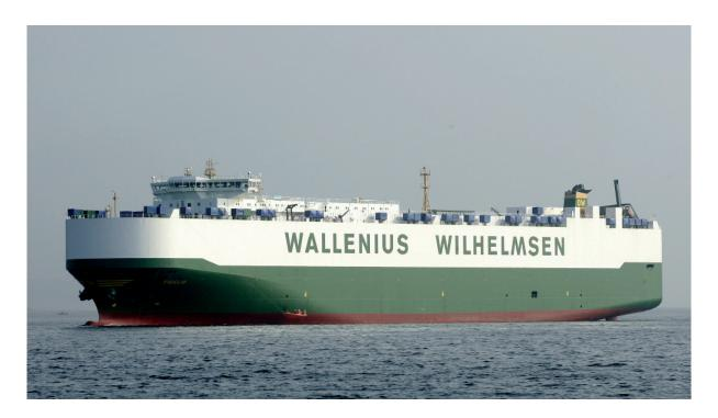
The LCTC (Large Car Truck Carrier) m/v FIDELIO has a capacity of 8,000 cars or a combination of 3,484 cars and 468 buses. With her 227.8 metres this capacity makes her one of the largest car carriers in the world. The vessel is built to the highest class of Lloyd's Regis-
